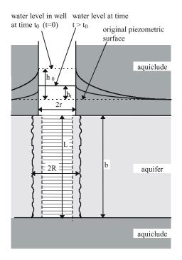
Hvorslev defined the *time lag*,  $T_L$  (the time required for the initial pressure change induced by the injection/extraction to dissipate, assuming a constant flow rate) as:
