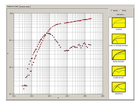
With the additional smoothing, the diagnostic graph clearly reveals double porosity aquifer conditions.
