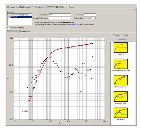
The graph can be further enhanced by increasing the **L-Spacing** of the derivative method.
