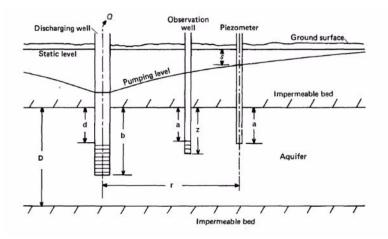
AquiferTest uses the vertical flow correction developed by Weeks (1969):
