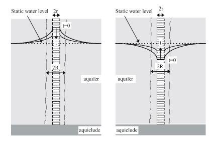
In cases where the water level drops within the screened interval, the plot of  $h/h_0$  vs. t will often have an initial slope and a shallower slope at later time. In this case, the fit should be obtained for the second straight line portion (Bouwer, 1989).
