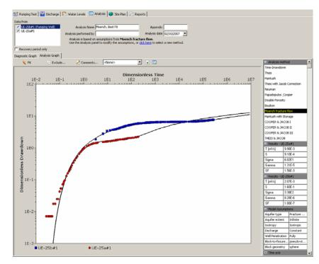
An example of a Moench Fracture Flow analysis is available in the project: AquiferTest\Examples\Moench Fracture Skin.HYT
