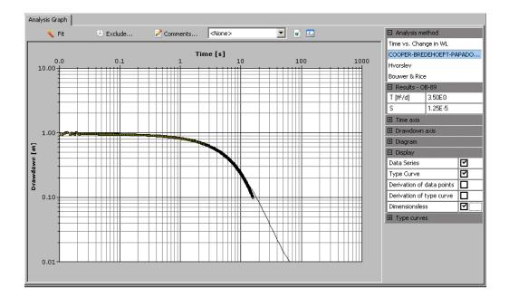
An example of a Cooper-Bredehoeft-Papadopulos slug test is available in the project: AquiferTest\Examples\SlugTest1.HYT.
