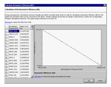
The dialog displays a graph with the data and fits a line – and calculates the BE value.
