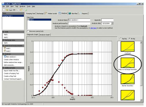
In the Semi-Log plot, you can compare the observed drawdown curve to the diagnostic plots. In this example, it is evident that the observed drawdown curve (outlined in the image above) is very similar to that expected in a Leaky aquifer (refer to the theoretical drawdown curve in the second diagnostic graph, circled above). For more details on the diagnostic graphs, see Chapter 4: Diagnostic Plots.
