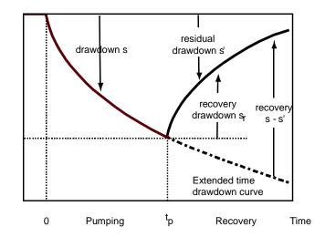
Agarwal defines the recovery drawdown  $s_r$  as the difference between the head h at any time during the recovery period and the head  $h_p$  at the end of the pumping period.
