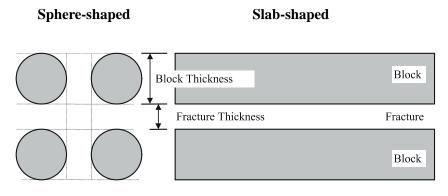
Moench (1984) uses the existence of a fracture skin to explain why well test data support both the pseudo-steady-state and transient block-to-fracture flow methods. The fracture skin is a thin skin of low permeability material deposited on the surface of the blocks, which impedes the free exchange of fluid between the blocks and the fissures.
