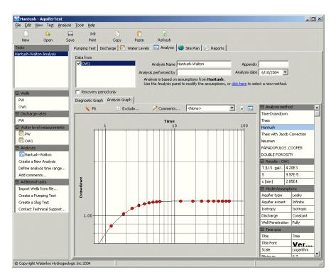
In this example, the dimensionless view is shown. An example of a Hantush-Jacob analysis is available in the project: AquiferTest\Examples\Leaky.HYT.
