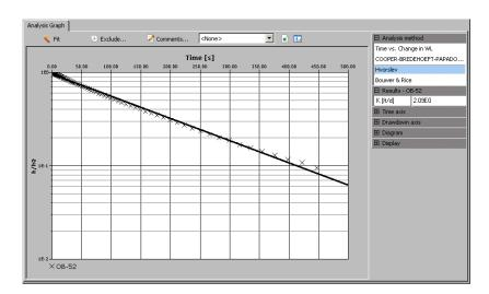
An example of a Hvorslev slug test is available in the project: AquiferTestAquiferTest\Examples\SlugTest2.HYT.
