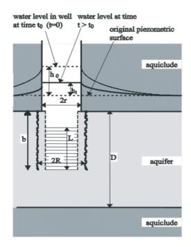
Bouwer-Rice (1976) developed an equation for hydraulic conductivity as follows:
