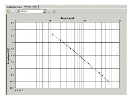
In this example, the time data is plotted on a logarithmic axis, and the drawdown axis is linear.
