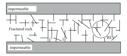
There are two double porosity models used in AquiferTest, which have been widely accepted in the literature. These are the pseudo-steady-state flow (Warren and Root, 1963) and the transient block-to-fracture flow (for example, Kazemi, 1969).
