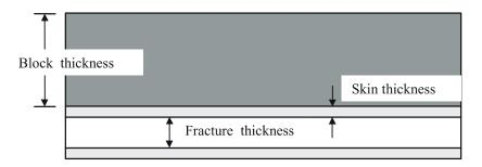
If the fracture skin is sufficiently impermeable, most of the change in hydraulic head between the block and the fracture occurs across the fracture skin and the transient blockto-fracture flow solution reduces to the pseudo-steady-state flow solution.
