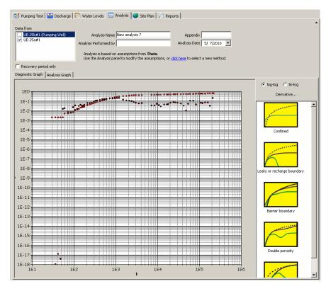
As you can see this diagnostic plot does not really give a clear indication of conditions of the aquifer system, *i.e.*, it cannot be easily matched to one of the diagnostic plot templates.
