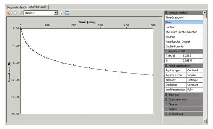
[21] To modify the plot axes, expand the **Display** frame of the **Analysis Navigator** panel and check the box beside **Dimensionless**
