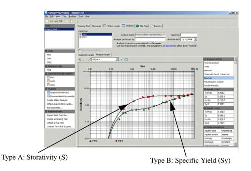
In this example, the dimensionless view is shown. An example of a Neuman analysis is available in the project: AquiferTest\Examples\PartiallyPenetratingWells.HYT.
