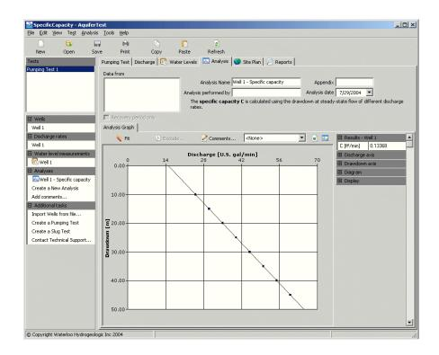
An example of a Specific Capacity analysis is available in the project: AquiferTest\Examples\SpecificCapacity.HYT.
