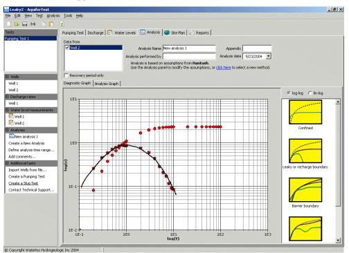
In this image, you can see the observed drawdown data, and the calculated derivative data. The derivative data is distinguished by an X through the middle of each data symbol, and is delineated in the image above.
