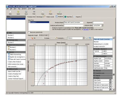
In this example, the dimensionless view is shown. An example of a Theis (Jacob Correction) analysis is available in the project: AquiferTest\Examples\Unconfined.HYT.
