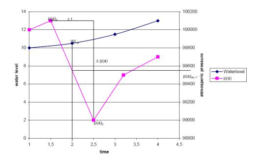
In the figure above you can see how **AquiferTest** will interpolate the atmospheric pressure p(a) for the time of water level measurement WL2 at t=2 where no value for p(a) is available.
