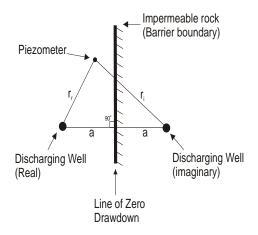
The cross-sectional view of the Stallman Barrier condition is seen below:
