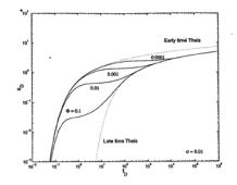
The following image displays a diagnostic plot of Boulton (1963) type curve
