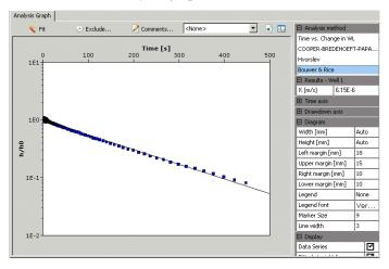
An example of a Bouwer & Rice slug test is available in the project: AquiferTest\Examples\SlugTest1.HYT.
