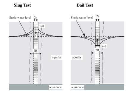
In cases where the water level drops within the screened interval, the plot of  $h_t/h_0$  vs. t will often have an initial slope and a smaller slope at later time (known in the literature as the 'double straight line effect'). In this case, you should manually fit the line to the second straight-line portion of the data (Bouwer, 1989). It is not necessary for the line to go through (1,0).
