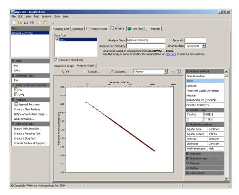
In this example, only the recovery data is displayed. An example of an Agarwal recovery solution is available in the project: AquiferTest\Examples\Agarwal-Recovery.HYT.
