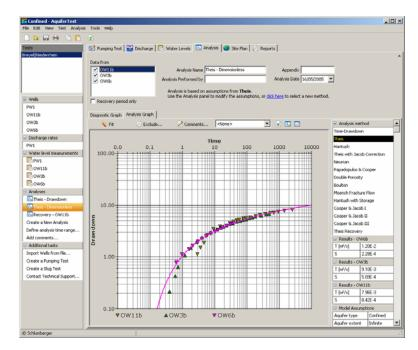
In this example, the dimensionless view is shown. An example of a Theis analysis is available in the project: AquiferTest\Examples\Confined.HYT.
