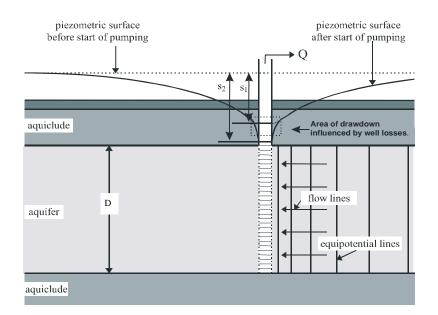
The figure above illustrates a comparison between the theoretical drawdown in a well (S1) and the actual drawdown in the well (S2) which includes the drawdown components inherent in S1 but also includes additional drawdown from both the linear and non-linear well loss components.
