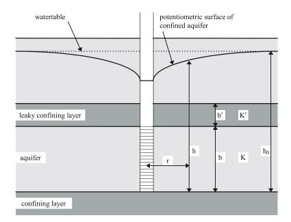
In the case of leaky aquifers, the well function W(u) can be replaced by the function Walton W(u, r/L) or Hantush W(u, B), and the solution becomes:
