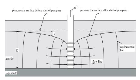
The equation developed by Neuman representing drawdown in an unconfined aquifer is given by:
