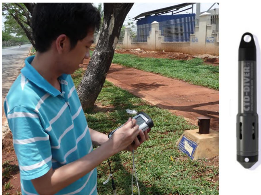
Figure 3. CTD Diver by Schlumberger Water Services is read out on the spot by Mr. Thang
